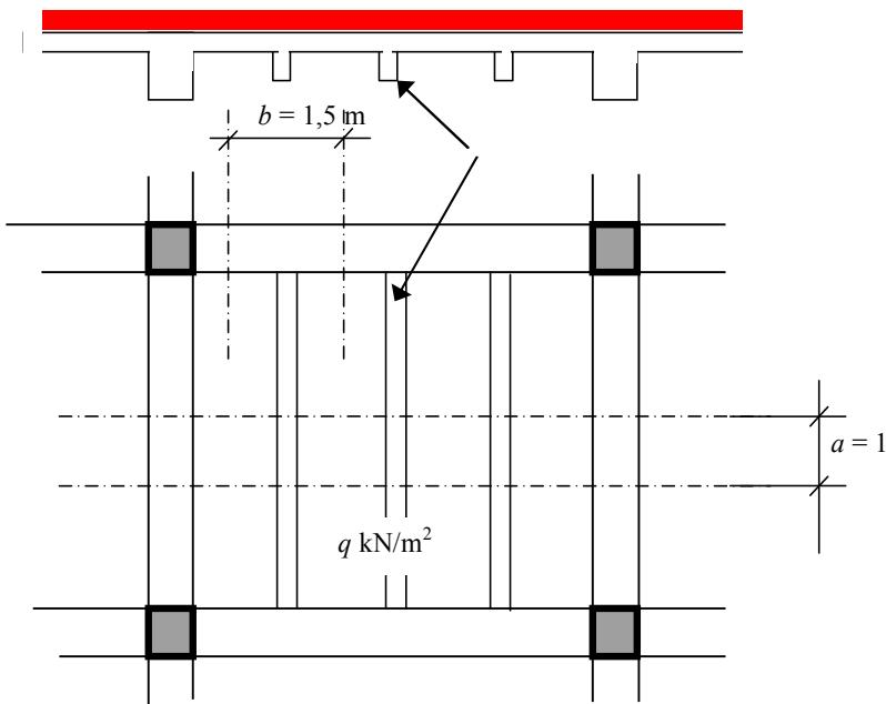
Determine action on the beam for verification of the ultimate limit state. Axial distance of the beams is 1 to 2 m, cross section dimensions  $0,45 \times 0,20 \text{ m}$  (including the slab thickness), slab thickness is 0,1 m. Consider the permanent load due to slab (volume weight is  $25 \text{ kN/m}^3$ ) and imposed load  $q_k = 1,50 \text{ kN/m}^2$ . Partial factor for the permanent and imposed loads are  $\gamma_G = 1,35$  and  $\gamma_Q = 1,5$ .
