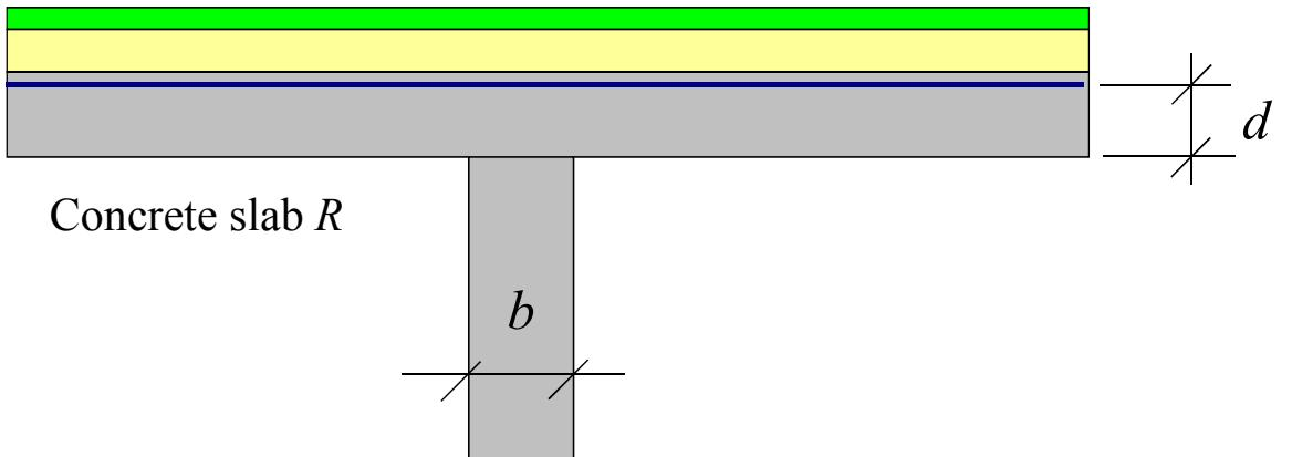
Verify resistance of the flat slab exposed to permanent load due to permanet load  $g_k = 7 \text{ kN/m}^2$  and imposed load  $q_k = 5 \text{ kN/m}^2$  ( $\gamma_G = 1,35$ ,  $\gamma_Q = 1,5$ ). Consider loading area  $36 \text{ m}^2$ . The effective depth of the slab is  $d = 0,15 \text{ m}$ , design shear strength  $\tau_c = 2 \text{ MPa}$ . The slab is supported by a circular column of the diameter  $b = 0,30 \text{ m}$ .
