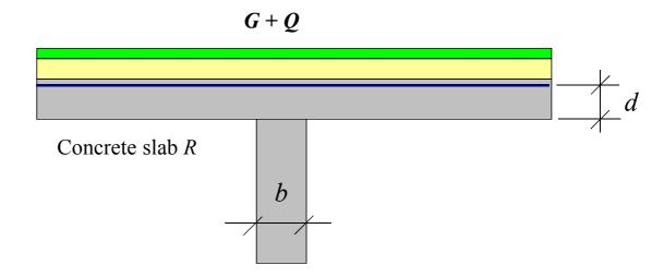
Verify resistance of the flat slab exposed to permanent load due to permanet load  $g_k = 7 \text{ kN/m}^2$  and imposed load  $q_k = 5 \text{ kN/m}^2$  ( $\gamma_G = 1,35$ ,  $\gamma_Q = 1,5$ ). Consider loading area 36 m². The effective depth of the slab is d = 0,15 m, design shear strength  $\tau_c = 2$  MPa. The slab is supported by a circular column of the diameter b = 0,30 m.
