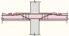
However, the **bottom bars**, being more deeply embedded, are not pushed out in the same way and thus provide more resistance. This is attributable initially to **dowel** action, and then later at larger deformations to its being **kinked**, as shown.
