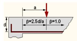
The formula for shear capacity,  $\tau_c = \tau_{Rd} k (1.2 + 40 \rho_l) + |\underline{0.15}| \sigma_{cp}$  makes no allowance for the increased shear strength for small values of ald at <u>direct supports</u>, where there is a clear strut or arch action.
