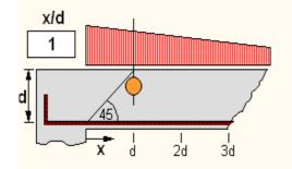
For continuous distributed loading, as indicated by the shear force diagram, the shear capacity is unchanged. Instead a reduction in shear force is generally effected by not considering the design shear force nearer than an effective depth, d from the face of a direct support.
