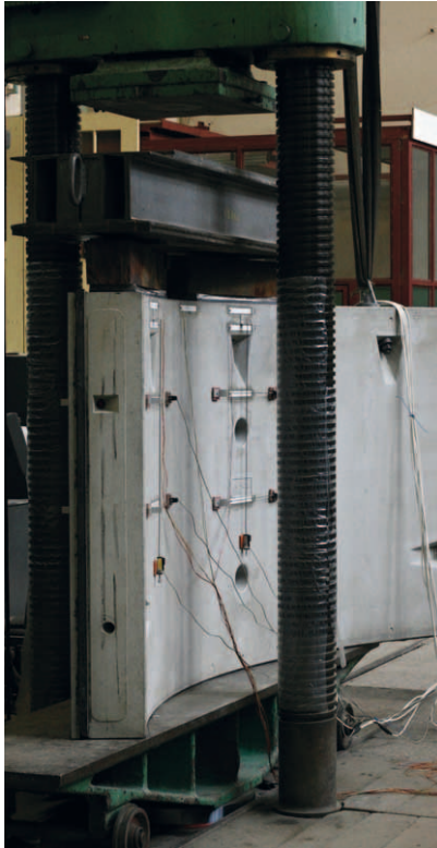
Test of a panelling segment of the extension of Metro Line A in Prague
